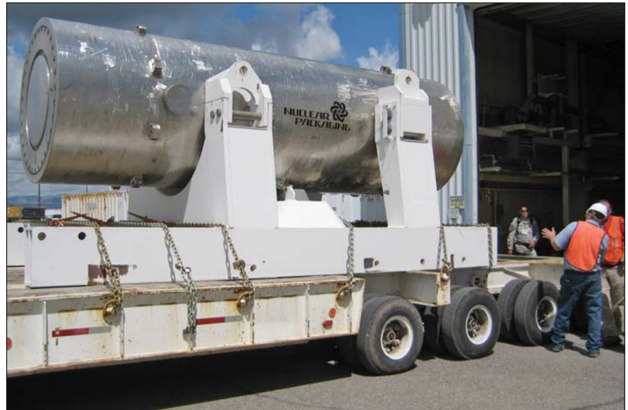
One of the NuPac 125-B casks is prepared for transport into a storage facility.
