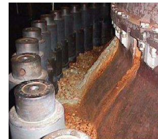
Red Rusty Ferric Acid Deposits on Vessel Flange (2RFO)
