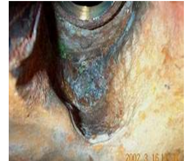
Red Rusty Ferric Acid Deposits on Vessel Flange (2RFO)
