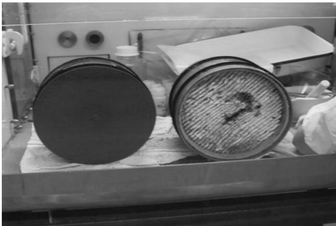
Figure 4 Glovebox HEPA following the incident
